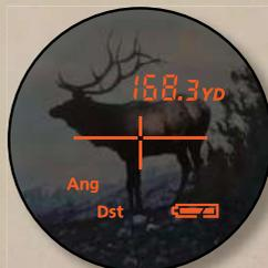
In darker conditions, the rangefinder will automatically turn on the orange LED illumination to the liquid crystal characters for optimum visibility—even adjusting its brightness as needed for appropriate contrast against the background.
